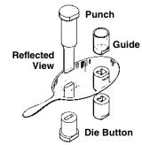
Note: Must identify as REFLECTED VIEW on punch drawing.
